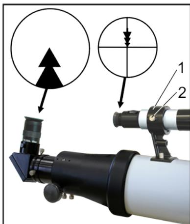
Telescope has high magnifications and consequently – small fields of view. This complicates the search of objects in the sky, that is why the telescope is equipped with an optical finder with a wide field of view. With the help of the finder you can easily find the necessary object in the sky and then observe it in the field of view of the telescope. For this purpose you should adjust the parallelism of the optical axes of telescope tube and optical finder.
